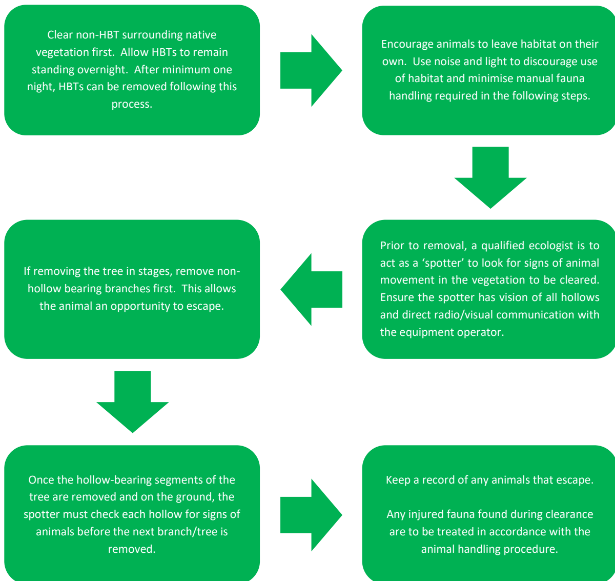
Figure 9-2: Hollow-bearing tree removal procedure
